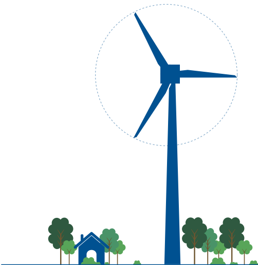
Wind Turbine 27m rotor Hub height 30m
